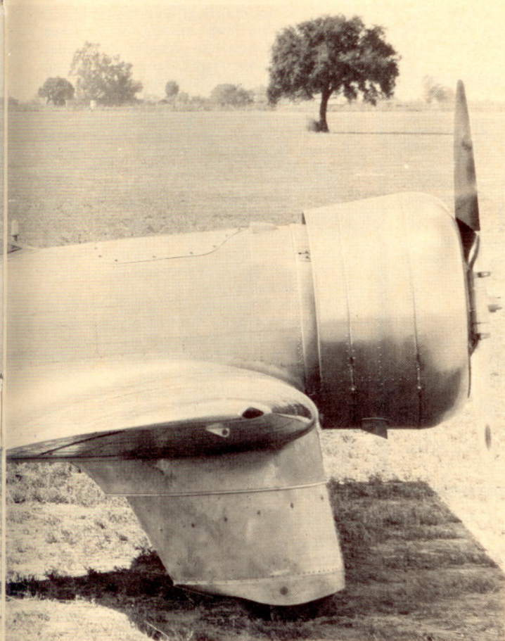
The second and final Beta was fitted with a 300-hp P&W Wasp Jr. engine. Note the closed-off front cockpit and the vertical tracks for the movable fairing between the horizontal stabilizer and the fuselage. The lower thrust line and larger propeller of the radial engine required a slightly longer landing gear than was used on the Menasco-powered model.
